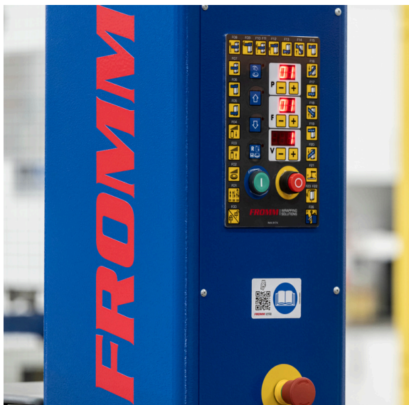
Operating Panel with 99 programs, emergency stop and reset buttons
